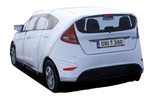
The Soft Car 360 is a lightweight, durable, and collapsible whole vehicle target that serves as the perfect ADAS testing solution when paired with a VRU platform.
